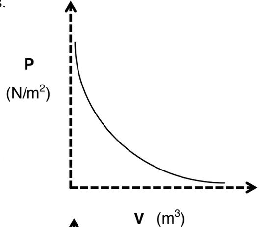
The curve appears to be a hyperbola (inverse function). Hyperbolic or inverse functions suggest a test plot be made of  $P$  vs  $\frac{1}{V}$ . The resulting graph is shown below:
