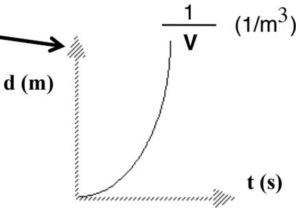
The curve appears to be a top-opening parabola. This function suggests that a test plot be made of  $d$  vs.  $t^2$ . The resulting graph is shown below:
