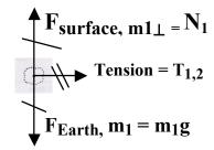
**Step 4 - Force equation for box 1 in X-direction (direction of acceleration)**
