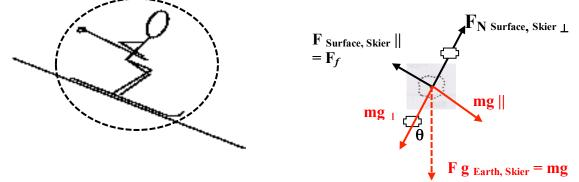
$$F_{f} = \mu * F_{N} \qquad F_{N} = mg \cos (\theta) = 60 \text{ kg} * 10 \text{ N/kg} * \cos (35^{\circ}) = 491 \text{ N}$$
