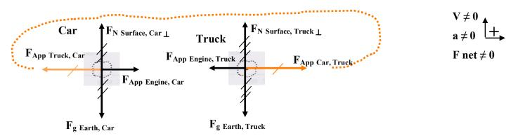
Since they are Newton's 3<sup>rd</sup> law paired forces they must be equal in size, but opposite in direction. Sizes of the paired forces does not depend on if an object accelerates.
