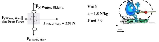
$\Sigma F = ma$  $F_{T Boat, Skier} - Drag Force = ma$ 220 N - Drag = 80 kg \* 1.8 N/kgDrag = 220 N - 80 kg \* 1.8 N/kgDrag = 220 N - 144 NDrag = 76 N
