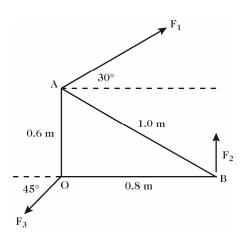
4. A light triangular plate OAB is in a horizontal plane. Three forces,  $F_1 = 2 \text{ N}$ ,  $F_2 = 4 \text{ N}$ , and  $F_3 = 7 \text{ N}$ , act on the plate, which is pivoted about a vertical axis through point O. In the figure, consider the counterclockwise sense as positive. The sum of the torques about the vertical axis through point O, acting on the plate due to forces  $F_1$ ,  $F_2$ , and  $F_3$ , is closest to:
