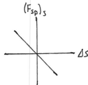
11. A spring has an unstretched length of 10 cm. It exerts a restoring force  $F$  when stretched to a length of 11 cm.
