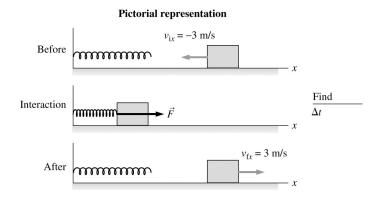
**Solve:** Using the impulse-momentum theorem  $p_{fx} - p_{ix} = \int F(t) dt$ ,
