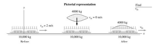
**Solve:** There are no *external* horizontal forces on the car + gravel system, so the horizontal momentum is conserved. This means  $p_{fx} = p_{ix}$ . Hence,
