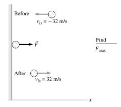
The force increases to  $F_{\text{max}}$  during the first two ms, stays at  $F_{\text{max}}$  for two ms, and then decreases to zero during the last two ms. The graph shows that  $F_x$  is positive, so the force acts to the right.
