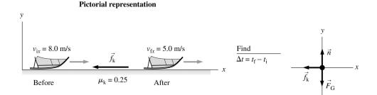
Note that the force of kinetic friction  $f_k$  imparts a negative impulse to the sled.
