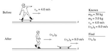
The system has nonzero initial momentum  $p_{ix}$ . As Dan (D) jumps backward off the gliding skateboard (S), the skateboard will move forward so that the final total momentum of the system  $p_{fx}$  is equal to  $p_{ix}$ .
