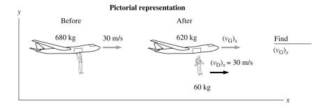
Note that there are no *external* forces in the *x*-direction (ignoring friction in the impulse approximation), implying conservation of momentum along the *x*-direction.
