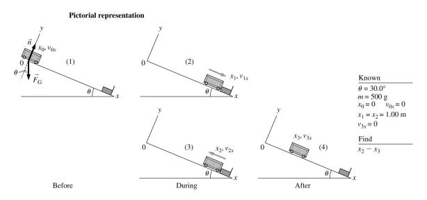
Solve: From the free-body diagram on the cart, Newton's second law applied to the system before the collision gives
