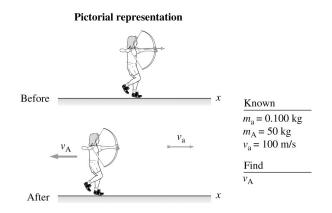
The initial momentum  $p_{ix}$  of the system is zero, because the archer and the arrow are at rest. The final moment  $p_{fx}$  must also be zero.
