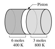
Is the pressure in the gas on the left side (i) greater than, (ii) less than, or (iii) equal to the pressure in the gas on the right side? \_\_\_\_\_
