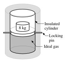
If the piston moves upward the gas will have done work on the piston and metal cylinder, and if it moves downward there will be work done on the gas by the piston and cylinder. In either case, the internal energy of the gas changes, which corresponds to a change in the temperature of the gas. The insulated cylinder prevents energy exchange between the gas and the environment via heating, but this alone does not prevent a change in temperature.
