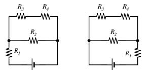
Will the potential difference across  $R_1$  be (i) *larger* in the circuit on the left, (ii) *smaller* in the circuit on the left, or (iii) *equal* in both? \_\_\_\_\_ Explain your reasoning.
