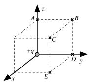
Rank the strength (magnitude) of the electric force on a +3q point charge if it is placed at the labeled points.
