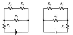
Will the current in  $R_1$  be (i) *larger* in the circuit on the left, (ii) *smaller* in the circuit on the left, or (iii) *equal* in both circuits? \_\_\_\_\_ Explain your reasoning.
