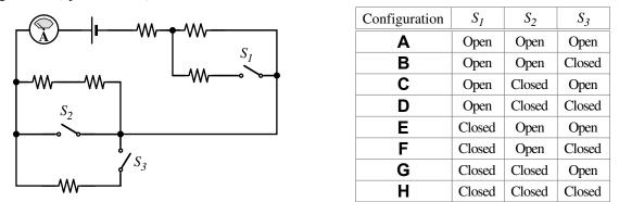
Rank the current in the ammeter for these switch configurations.
