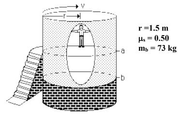
Determine the period of rotation necessary to keep the riders from sliding down the wall when the floor is lowered from point "a" to point "b". (Show all of your work and explain your reasoning.)
