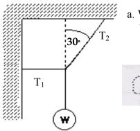
a. Write the equation for the sum of the forces in the x-direction. What is the value of  $T_2(F_{rope 2, box})$ ?
