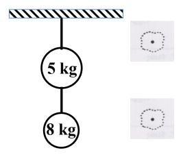
3. The object hung from the cable has a weight of 50 N. Write the equation for the sum of the forces in the y-direction. What is the tension  $(F_{Tension})$  in the cable?
