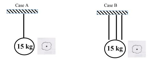
2. Determine tension in each cable. (Hint: There is more than one way to define the system.)
