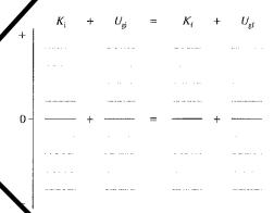
7. A ball starts from rest on the top of one hill, rolls without friction through a valley, and just barely makes it to the top of an adjacent hill.
