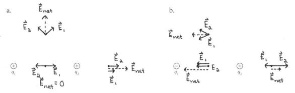
6. For each of the figures, use dots to mark any point or points (other than infinity) where  $\vec{E} = \vec{0}$ .
