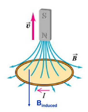
Let's consider a magnet with it's north pole moving AWAY from a conducting loop.
