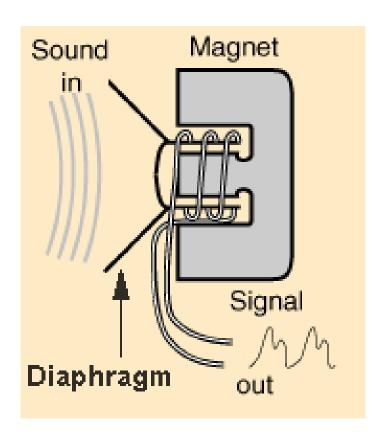
A microphone works when sound waves enter the filter of a microphone. Inside the filter, a diaphragm is vibrated by the sound waves which in turn moves a coil of wire wrapped around a magnet. The movement of the wire in the magnetic field induces a current in the wire. Thus sound waves can be turned into electronic signals and then amplified through a speaker.
