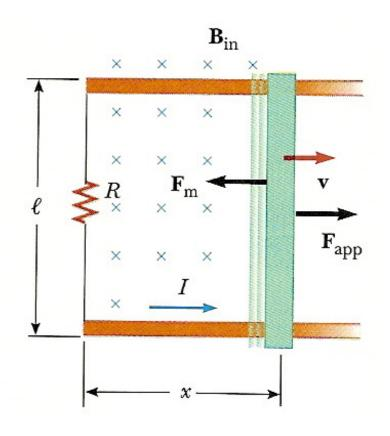
In the figure, we are applying a force this time to the rod. Due to Lenz's Law the magnetic force opposes the applied force. Since we know that the magnetic force acts to the left and the magnetic field acts into the page, we can use the RHR to determine the direction of the current around the loop and the resistor.
