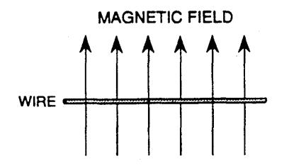
A 36-m length wire carries a current of 22A running from right to left. Calculate the magnitude and direction of the magnetic force acting on the wire if it is placed in a magnetic field with a magnitude of 0.50 x10<sup>-4</sup> T and directed up the page.
