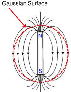
But if we enclose a MAGNET, we have the same # of magnetic field lines entering the closed surface as we have leaving, thus the NET MAGNETIC FLUX = ZERO!
