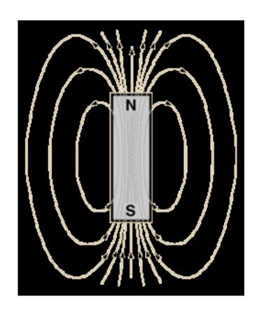
A bar magnet has a magnetic field around it. This field is 3D in nature and often represented by lines LEAVING north and ENTERING south
