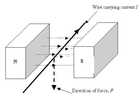
You simply used the RIGHT HAND ONLY and the thumb will represent the direction of the CURRENT instead of the velocity.
