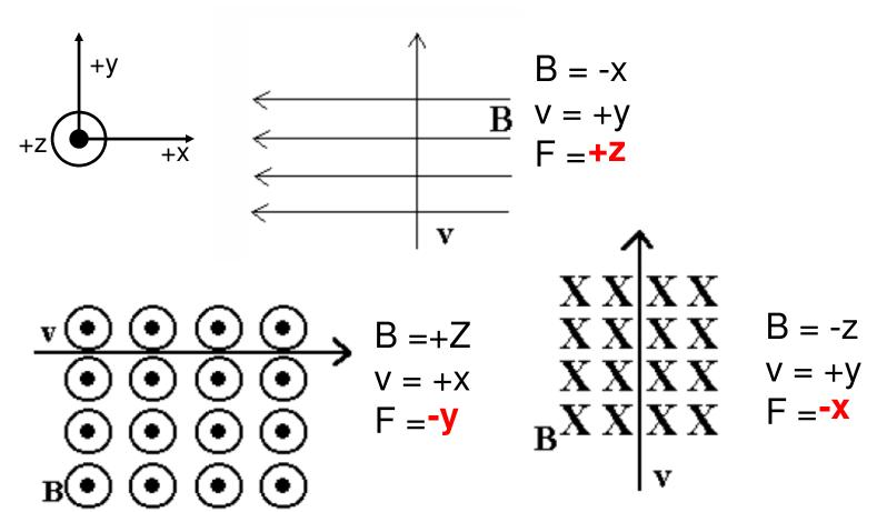
Determine the direction of the unknown variable for an electron using the coordinate axis given.
