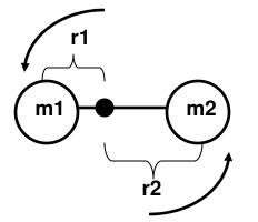
Since it is a rigid body, the have the SAME angular velocity,  $\omega$ . The velocity of the center,  $v_{cm}$  of mass is zero since it is rotating around it. We soon see that the TANGENTIAL SPEEDS are NOT EQUAL due to different radii.
