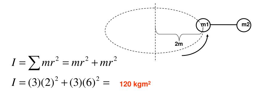
As you can see, the FARTHER the axis of rotation is from the center of mass, the moment of inertia increases. We need an expression that will help us determine the moment of inertia when this situation arises.
