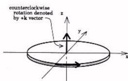
**Example: Unscrewing a screw or bolt**
