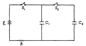
1975E2. In the diagram above, V = 100 volts;  $C_1 = 12$  microfarads;  $C_2 = 24$  microfarads; R = 10 ohms. Initially,  $C_1$  and  $C_2$  are uncharged, and all switches are open.
