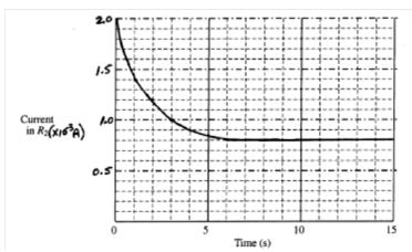
The energy would be greater. Consider the circuit a long time after the switch is closed, when there is no f. current in the capacitor. If  $R_2$  is replaced with a smaller resistance, then the total resistance decreases. This results in a larger current through the resistors. Therefore, the voltage across  $R_1$ , and thus across the capacitor, increases.
