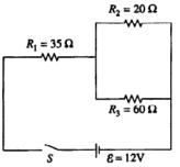
35. In the circuit shown above, the equivalent resistance of the three resistors is (A) 10.5  $\Omega$  (B) 15 $\Omega$  (C) 20  $\Omega$  (D) 50  $\Omega$  (E) 115  $\Omega$
