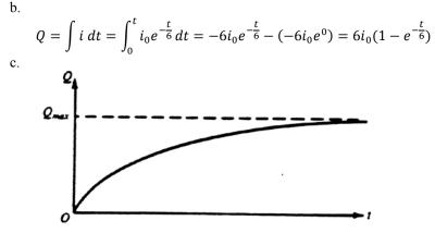
d. For charging a capacitor, the time constant is RC. The numerical value of the time constant is 6 seconds so  $C = 6/R = 3 \times 10^{-6} F$
