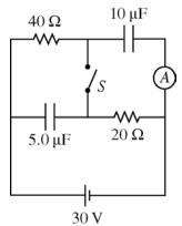
2010E2. In the circuit illustrated above, switch S is initially open and the battery has been connected for a long time.
