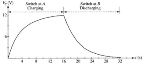
d. Draw a schematic diagram of the RC circuit that you constructed that would produce the graph above. Clearly indicate switch positions *A* and *B* on your circuit diagram and include whatever other devices you need to measure the voltage across the capacitor to obtain the above plot. Label each component in your diagram.
