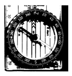
A long, straight current-carrying wire is brought close to the compass, deflecting the compass to the position shown above, 48° west of north.
