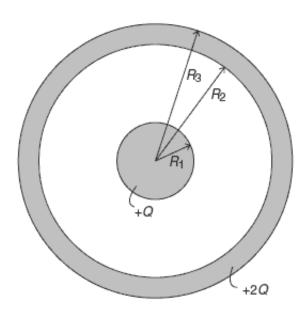
A metal sphere of radius  $R_1$  carries charge +Q. A concentric spherical metal shell, of inner radius  $R_2$  and outer radius  $R_3$ , carries charge +2Q.
