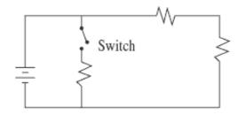
17. Three resistors are connected to a battery as shown in the diagram above. The switch is initially open. When the switch is closed, what happens to the total voltage, current, and resistance in the circuit?
