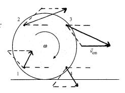
25. A wheel is rolling along a horizontal surface with the center-of-mass velocity shown. Draw the velocity vector  $\vec{v}$  at points 1 to 3 on the wheel.
