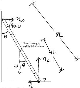
$$\begin{split} \mathcal{E}T_{p} &= T(3L) - \omega(4L)\sin(90+\theta) \qquad \mathcal{E}F_{x} &= N\omega - f_{F} = O \\ &-F_{R}(8L)\sin(90+\theta) \qquad \mathcal{E}F_{y} &= N_{F} - \omega = O \\ &= T(3L) - \omega(4L)\cos\theta - \omega(3L)\cos\theta = O \\ &= \Sigma T_{p} = \omega(4L)\sin\theta - N_{\omega}(8L)\sin\theta - O \\ &= \omega(4L)\sin\theta - N_{\omega}(8L)\cos\theta = O \end{split}$$
