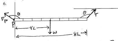
$\Sigma F_{X} = T_{X} + F_{PX} = T\cos\theta - F_{P}\cos\theta = 0$   $\Sigma F_{Y} = T_{Y} + F_{PY} - \omega = T\sin\theta + F_{P}\sin\theta - \omega = 0$   $\Sigma T_{P} = T\sin\theta(8L) - \omega(4L) = 0$
