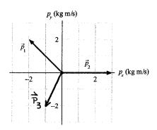
18. An object initially at rest explodes into three fragments. The momentum vectors of two of the fragments are shown. Draw the momentum vector  $\vec{p}_3$  of the third fragment.
