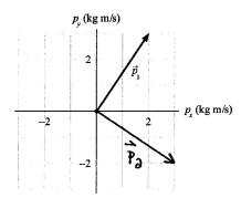
20. A 500 g ball traveling to the right at 4.0 m/s collides with and bounces off another ball. The figure shows the momentum vector  $\vec{p}_1$  of the first ball after the collision. Draw the momentum vector  $\vec{p}_2$  of the second ball.
