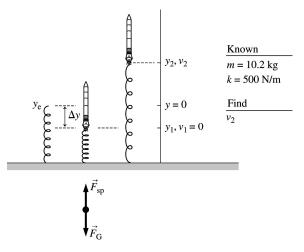
The origin of the coordinate system is placed on the free end of the spring. Note that the bottom of the spring is anchored to the ground.
