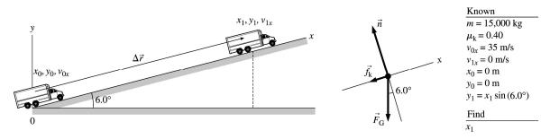
We place the origin of our coordinate system at the base of the ramp in such a way that the *x*-axis is along the ramp and the *y*-axis is vertical so that we can calculate potential energy. The free-body diagram of forces on the truck is shown.
