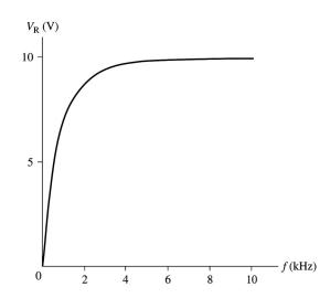
Assess: The circuit acts like a high-pass filter when the output voltage is taken across the resistor.
