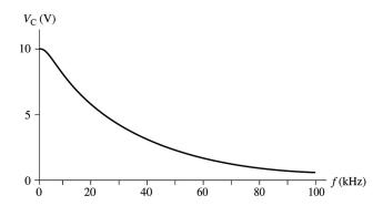
**Assess:** For the voltage across the capacitor, the circuit is a low-pass filter.
