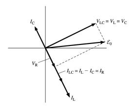
The capacitor and inductor currents add to give the phasor  $I_{LC} = I_L = I_C$ . The resistor is in series with the capacitor/inductor combination, and series elements share the same current, hence  $I_R = I_{LC}$ . For a resistor, the voltage  $V_R$  is in phase with the current  $I_R$ , and this has been shown on the diagram. Finally, the voltages  $V_R$  and  $V_{LC}$  add as vectors to give the emf voltage  $\mathcal{E}_0$ .
