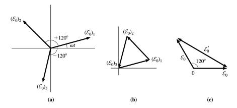
**Solve:** (a) The three phasors are shown in the figure above. The second phasor has a phase  $120^{\circ}$  ahead of the first and the third phasor has a phase that is  $120^{\circ}$  behind the first. These phasors are labeled as  $(\mathcal{E} \sim)1$ ,  $(\mathcal{E}_0)_2$ , and  $(\mathcal{E}_0)_3$ .
