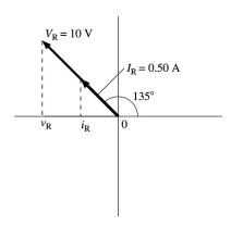
**Assess:** Ohm's law applies to both the instantaneous *and* peak currents and voltages. For a resistor, the current and voltage are in phase.
