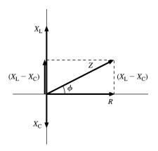
The figure above shows the nature of R,  $X_{\rm C}$ ,  $X_{\rm L}$ , and Z as a phasor diagram. The power factor is  $\cos\phi = 0.9$ . The total circuit impedance is found from  $Z = \mathcal{E}_{\rm rms}/I_{\rm rms} = (15,000 \text{ V})/(444 \text{ A}) = 33.8 \Omega$ . You can see from the right triangle in the diagram that
