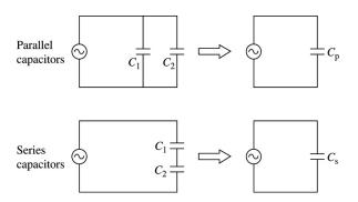
**Solve:** For a circuit with parallel capacitors,  $C_p = C_1 + C_2$ . The current in the circuit is
