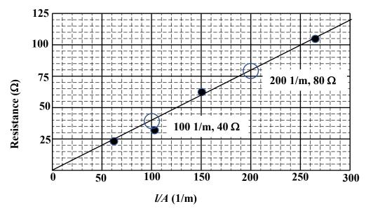
iii. Use the above graph to estimate a value for the resistivity of the dough cylinders.
